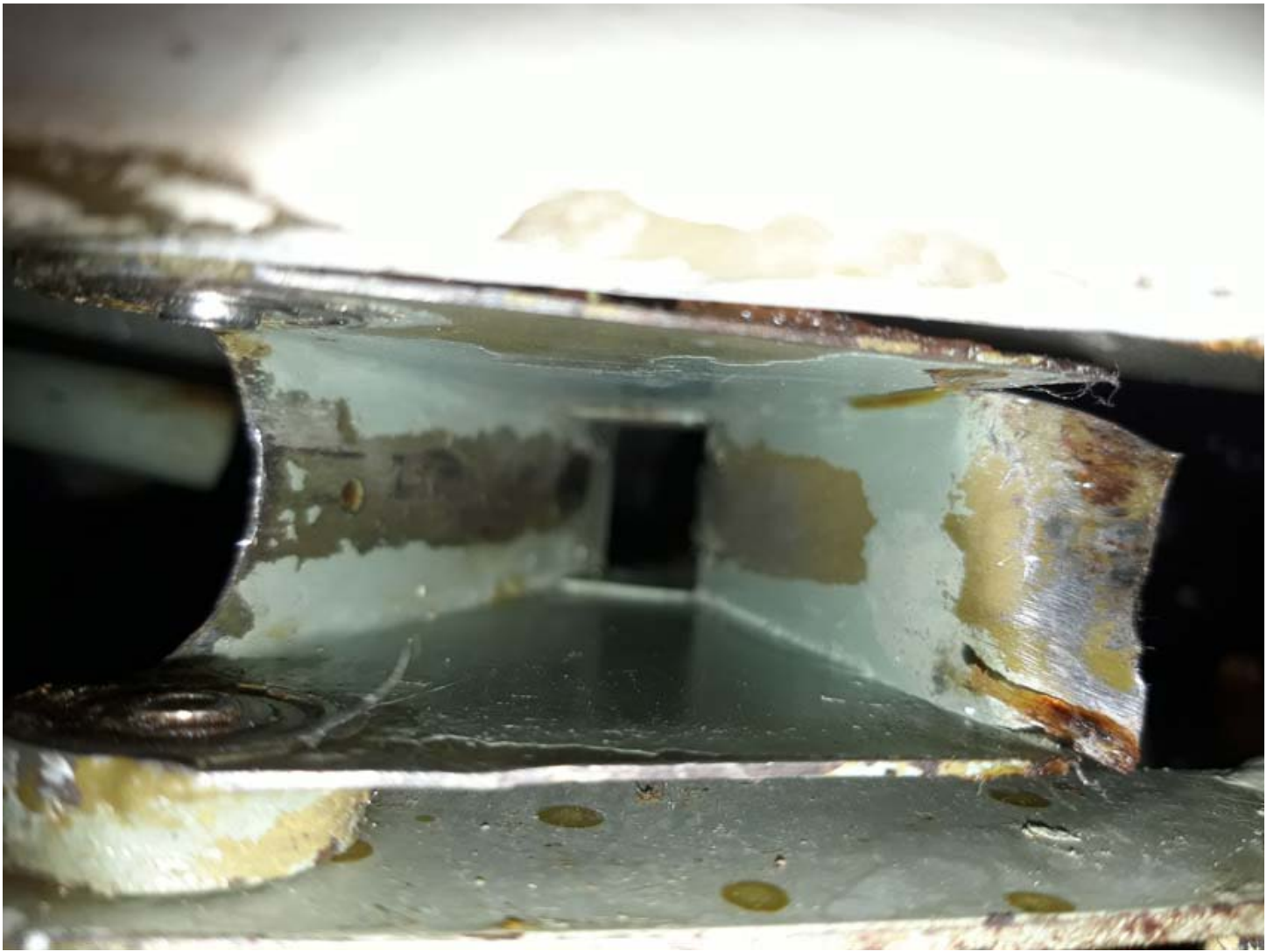
Rigging damage to the Vega – the funnels on both sides are the same.
