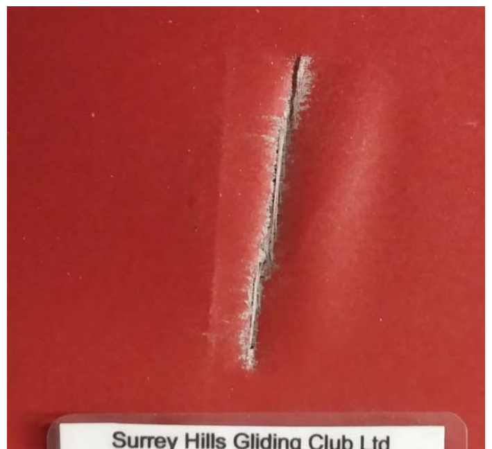
Damage to the K8 wing – a little carelessness.
